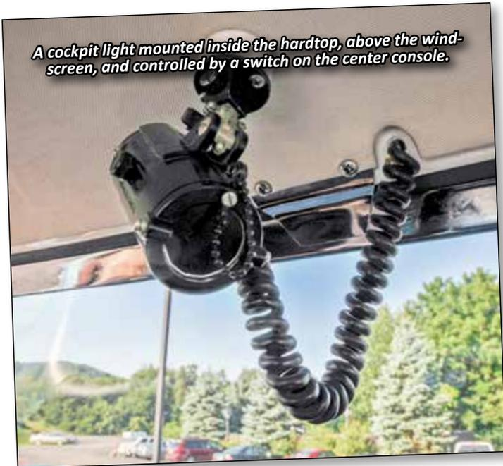
*A cockpit light mounted inside the hardtop, above the wind-screen, and controlled by a switch on the center console.*
