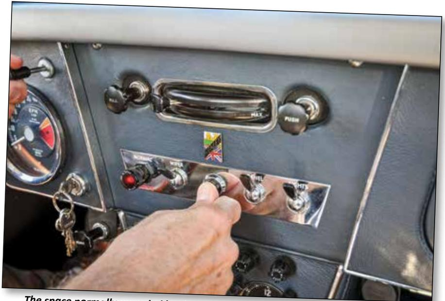
*The space normally occupied by the radio and speaker grille is now dedicated to compass, a clock, fuses and several switches. Note the ignition key at upper left where the windscreen washer button used to be, the overdrive switch on the gearshift knob, and the axillary power outlet at right.*
